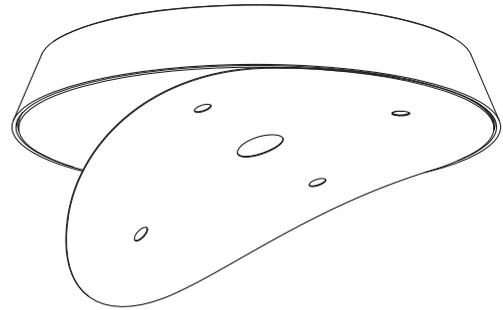
3 Ensure Surface is free from dirt or grease and install bezel.
